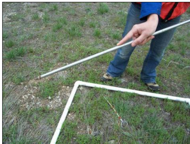
Figure 32. Read the number of inches the penetrometer rod penetrated into the soil by rounding up to the nearest inch. Each line on the penetrometer represents 3 inches. The reading here is 11 inches.
