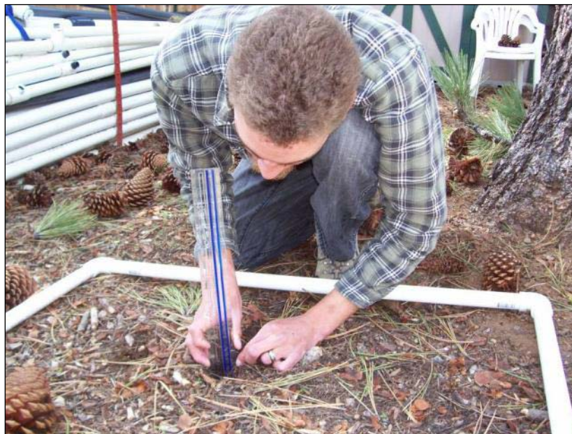
Figure 24. Conducting mulch depth measurements to the nearest ¼ inch. The mulch is brushed aside so that the ruler can be placed on the soil surface.
