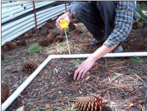
Figure 27. Spectrum Soil moisture meter, mulch is being brushed aside.
