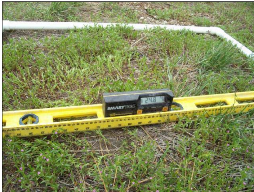
Figure 13. Digital level. Ensure that the digital level is on a level surface before taking the reading.
