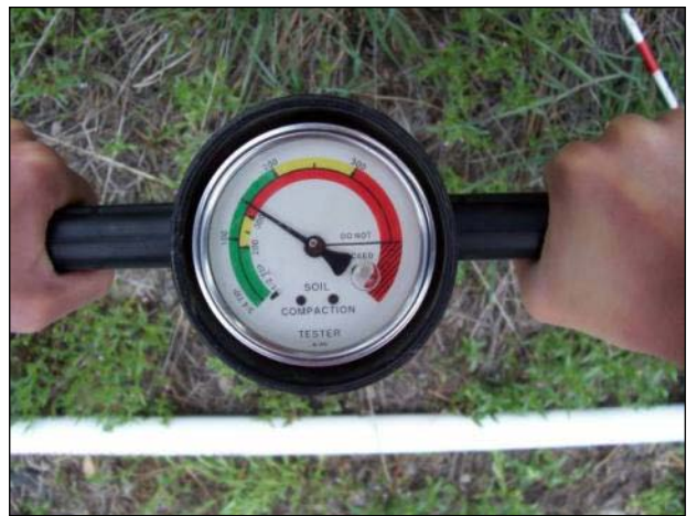
Figure 30. Penetrometer dial at 350 psi. Read the inner scale for the 1/2 inch tip.
