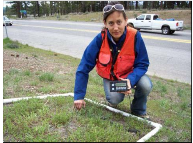
Figure 26. Hydrosense soil moisture meter in use. The probes are fully inserted into the soil.
