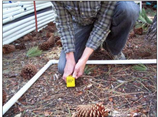
Figure 28. Spectrum soil moisture meter in use. The probe is inserted fully into the soil.
