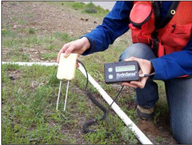
Figure 25. Hydrosense Soil Moisture Meter (sensor plus display)
