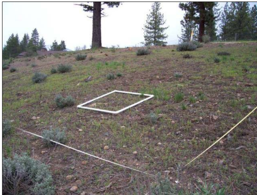
Figure 12. Quadrat (11ft 2 , 1m 2 ). The sub-area of interest is delineated with measuring tapes in this case. The area could also be marked by placing pin flags at the bottom corners of the sub-area.
